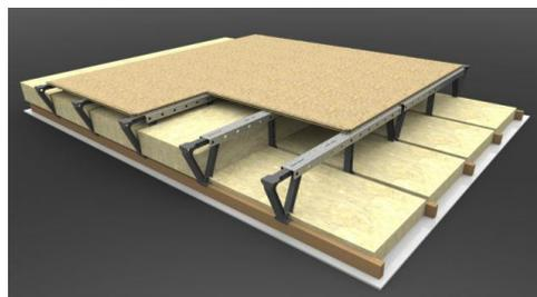
This will help distribute the weight more evenly across your loft ceiling adding support to your existing ceiling joists and raise the loft floor level to avoid compressing tall loft insulation.
